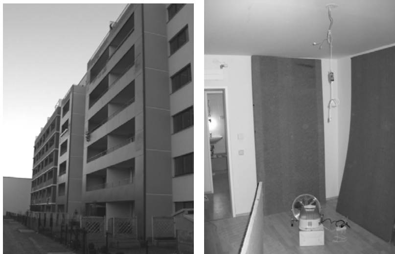
Fig 6 Apartment building in which a flat was provided for experimental purposes (left), and approximately 50m 2 , 2cm thick, soft fibreboard for increasing the moisture buffering effect of a room (right)
