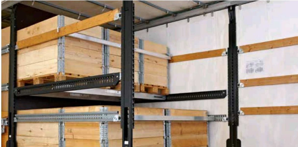
Figure: 2. Example of a solution to use the double flooring in the transport of general cargo
